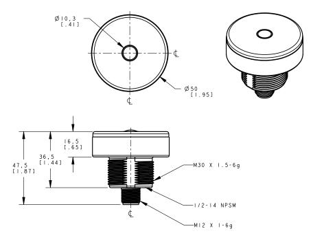
\* Push-button model shown. Push-button located in center of light.
