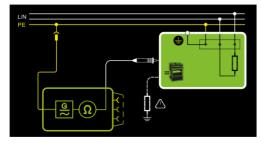
Test Function for Test Step in the Test Sequence
